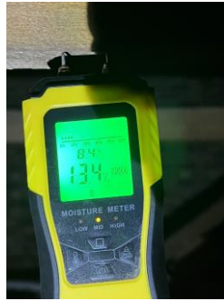
Timber moisture reading
