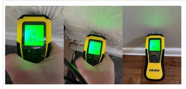
A damp reading was undertaken to the ground floor walls which showed a consistent, acceptable moisture reading level of 15 percent.
